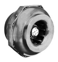
These models are named RS-(duct  $\emptyset$ ). The sizes RS-100L to RS-315L are equipped with an attractive, impact strong and hardly inflammable plastic casing with integrated IP-44 terminal box and guide vane. The impeller of the RS-315 is made of plastic. The impeller os the RS-315L is made of galvanized steel.
